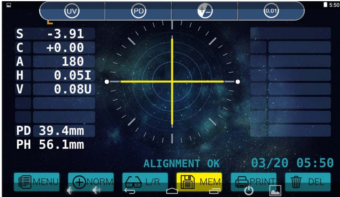
Figure 4.4 measurement of finished lens and save the data of left side
